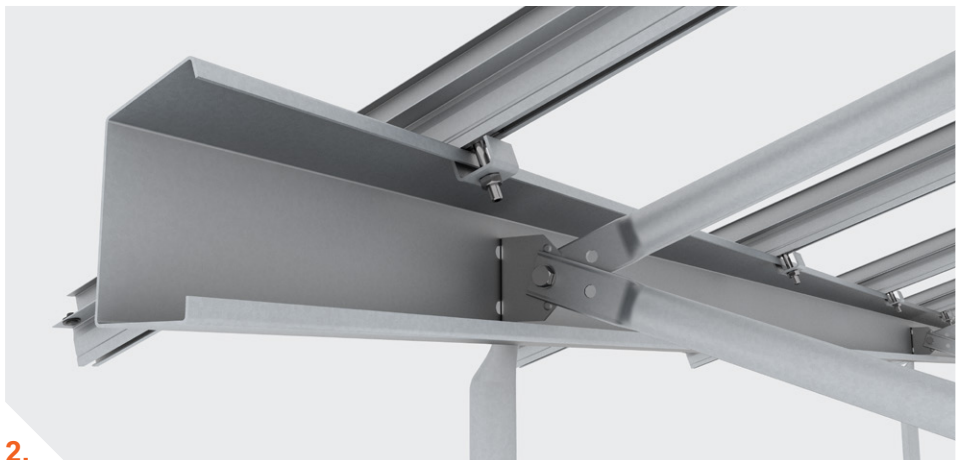
2. Attaching the bottom brace and the aluminum profile to the purlin, which determines the tilt of the panels
